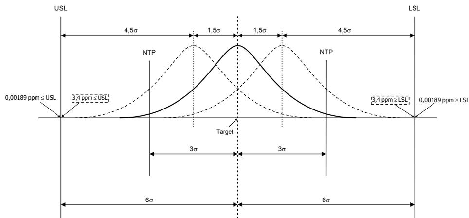
Figure 2. Statistical concept behind Six Sigma
